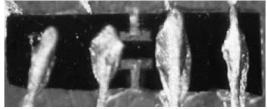
Fig. 2. The monocrystalline microbridge ( 200 \times 400 \mu\text{m}^2 ) of Bi-2212.
